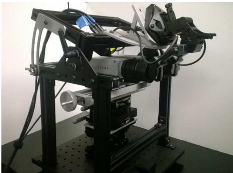
Proof of concept, deployable HMD measurement system developed by OBVA Lab.
